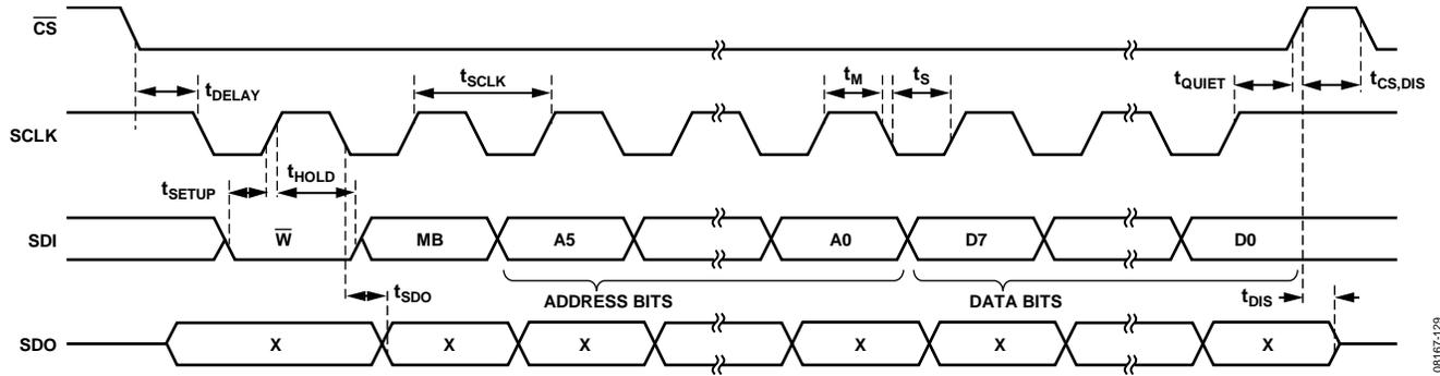
Figure 37. SPI 4-Wire Write
