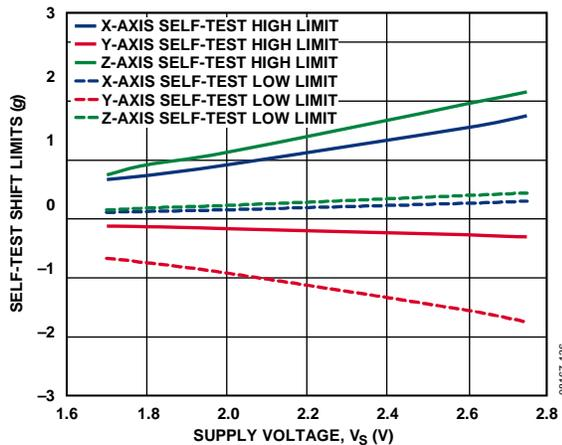
Figure 43. Self-Test Output Change Limits vs. Supply Voltage
