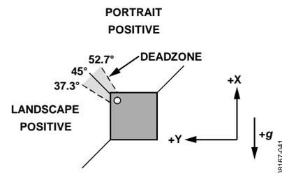
Figure 51. Orientation Showing a 15.4° Dead Zone Region
