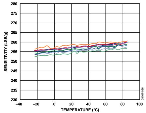
Figure 26. Y-Axis Sensitivity vs. Temperature—
