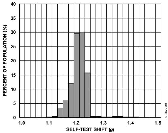
Figure 30. Z-Axis Self-Test Response at 25°C,  $V_S = 2.6 V$
