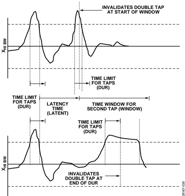
Figure 48. Tap Interrupt Function with Invalid Double Taps
