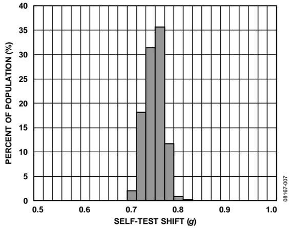
Figure 28. X-Axis Self-Test Response at 25°C,  $V_S = 2.6 V$
