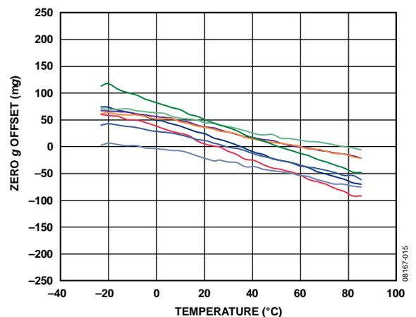
Figure 15. Z-Axis Zero g Offset vs. Temperature—
