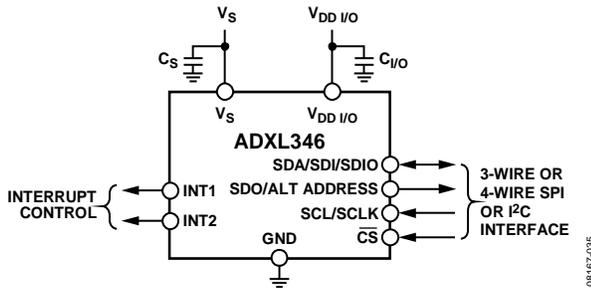
Figure 44. Applications Diagram
