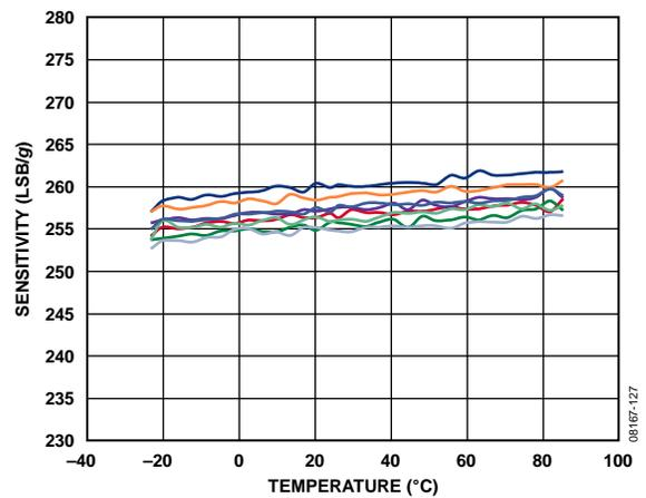
Figure 27. Z-Axis Sensitivity vs. Temperature—
