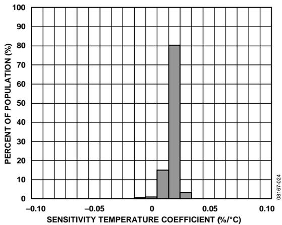
Figure 24. Z-Axis Sensitivity Temperature Coefficient,  $V_S = 2.6\text{ V}$
