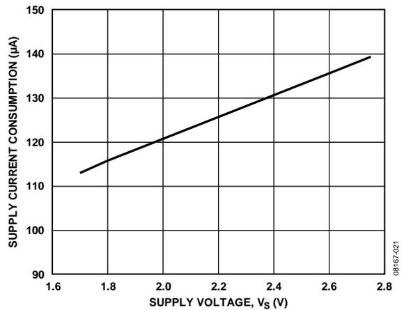
Figure 33. Supply Current vs. Supply Voltage at 25°C
