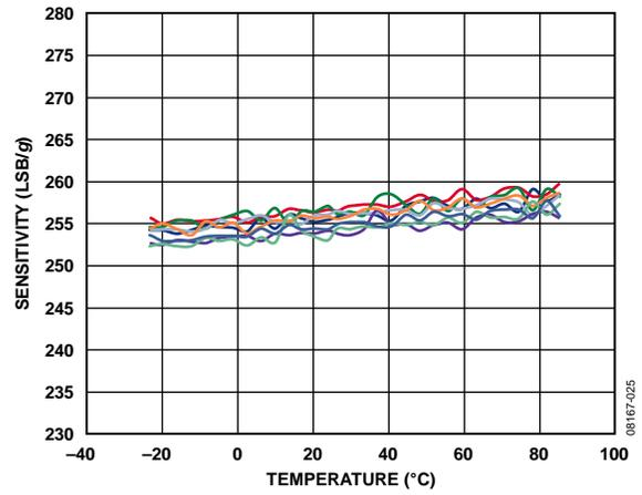
Figure 25. X-Axis Sensitivity vs. Temperature—
