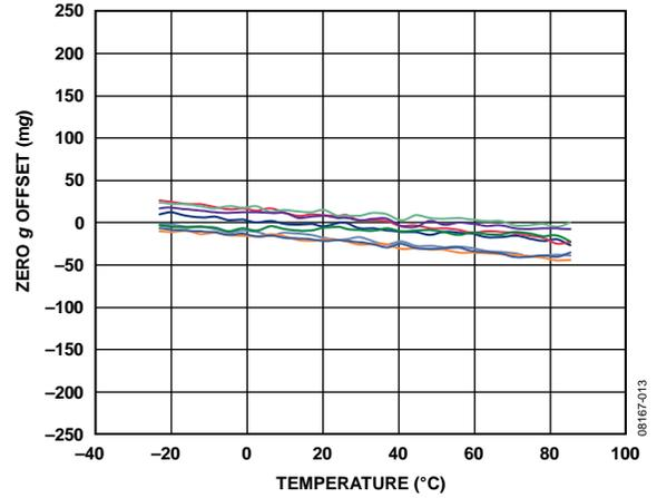
Figure 13. X-Axis Zero g Offset vs. Temperature—
