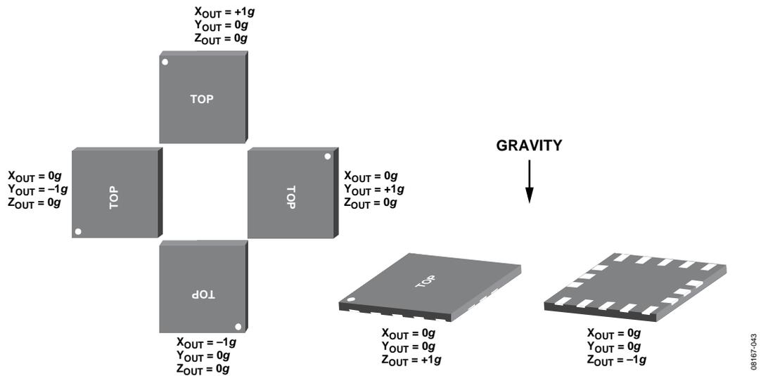
Figure 61. Output Response vs. Orientation to Gravity
