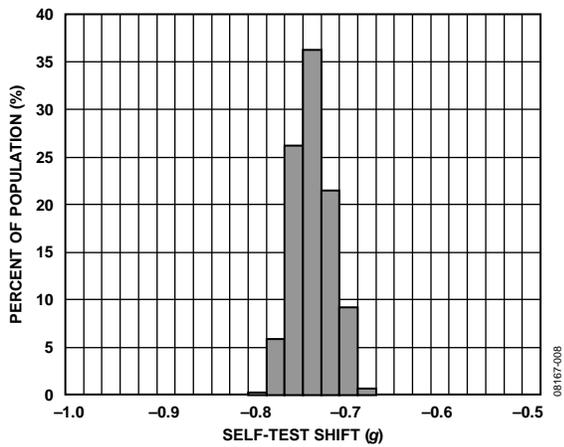
Figure 29. Y-Axis Self-Test Response at 25°C,  $V_S = 2.6 V$
