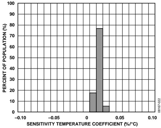
Figure 22. X-Axis Sensitivity Temperature Coefficient,  $V_S = 2.6\text{ V}$
