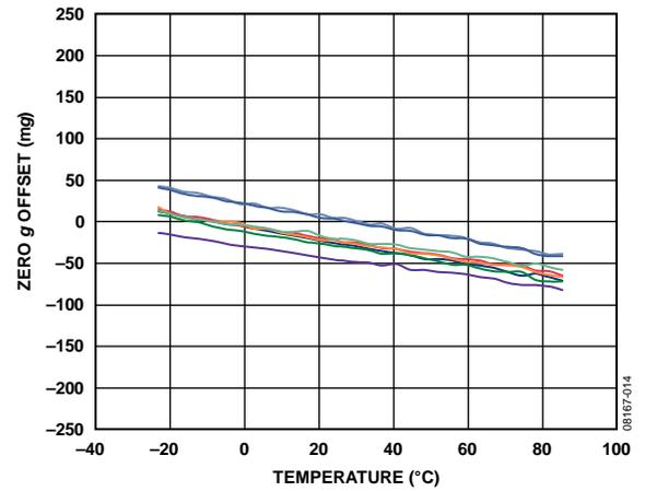
Figure 14. Y-Axis Zero g Offset vs. Temperature—
