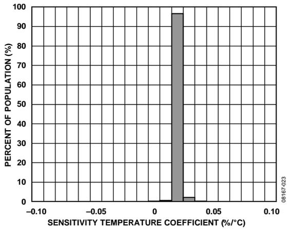
Figure 23. Y-Axis Sensitivity Temperature Coefficient,  $V_S = 2.6\text{ V}$
