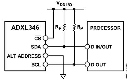
Figure 40. I<sup>2</sup>C Connection Diagram (Address 0x53)
