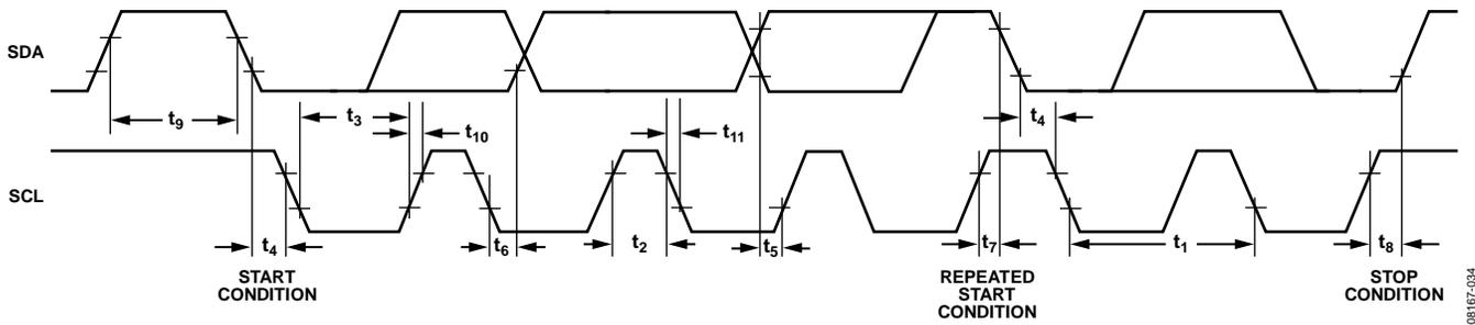
Figure 42. I<sup>2</sup>C Timing Diagram
